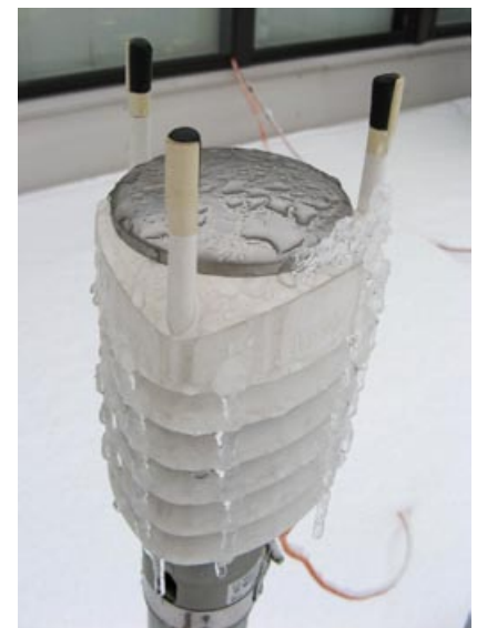
Heating at work in a WXT520.
