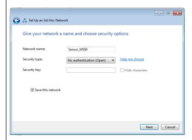
The new ad-hoc network will be established. Sometimes this does not work right away and several trials are needed. Always make sure that any other network connection (specially wireless) is off.
