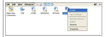
After that, tap again on OWL221A1 adapter and select Properties. On the WLAN adapter properties panel select Specify an IP address.
